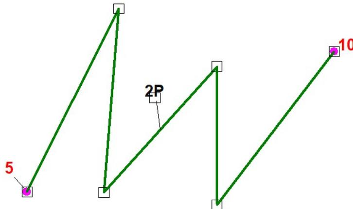
There is an option in the *Text Display Settings* to display Leader Lines for moved text items associated with pipes, nodes, or customers. If this option is selected (checked), when the associated text is moved, a leader line is automatically drawn between the text and the associated feature.
